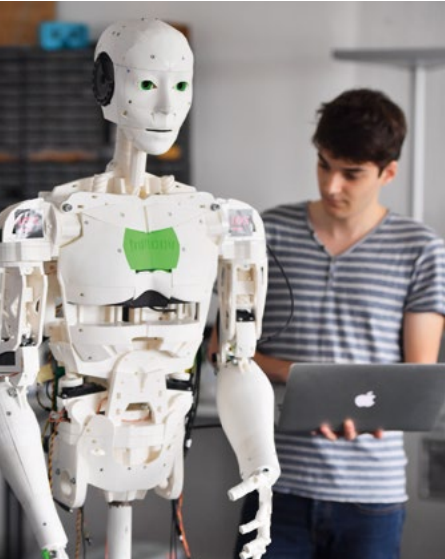
→ IOX LAB | The first humanoid robot completely made by 3-D printer
